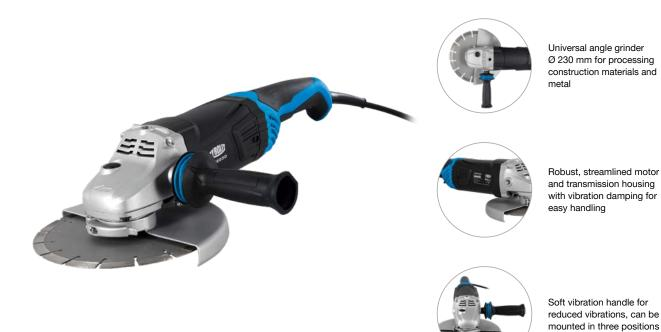
The AGE230 is a handy, streamlined Ø 230 mm angle grinder with vibration damping and longer handle, incl. a soft inlay for secure grip, a soft start feature and a blade guard that can be adjusted without tools. The robust steel transmission and a protected metal spindle bearing ensure reliability in use and a longer lifetime. As you would expect, this model has restart protection in case of power failure, a lock-on/off switch and a spindle lock.
