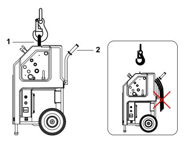
Fig. 8-1 Crane suspension shackle and transport handles
