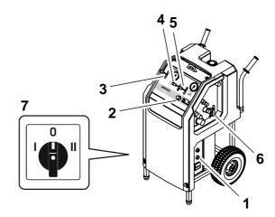
Fig. 5-3 Starting the Drive Unit PPH25\*\*
