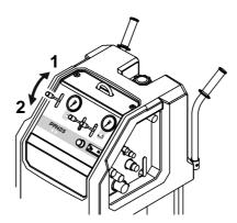
Fig. 5-4 Selecting the pressure stage
