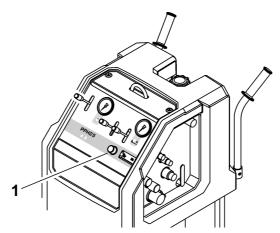
Fig. 5-6 Pressure control valve
