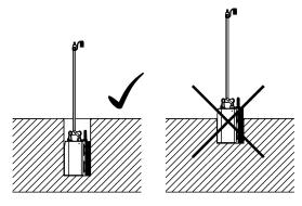
Fig. 4-1 Use in pocket bore holes
