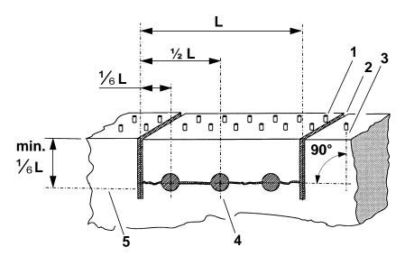
Fig. 4-5 Correct positioning when three pressing tools are used
