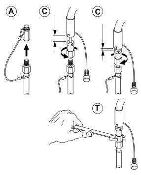
Fig. 3-8 Screw connection
