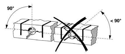
Fig. 4-3 Use at the correct angle
