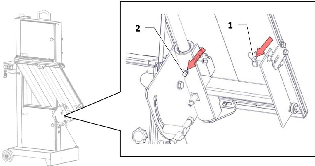
Lubrication points on the masonry band saw:
