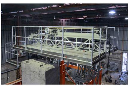
Large, stationary wire saws for the nuclear industry, developed by Studio Corvi.
